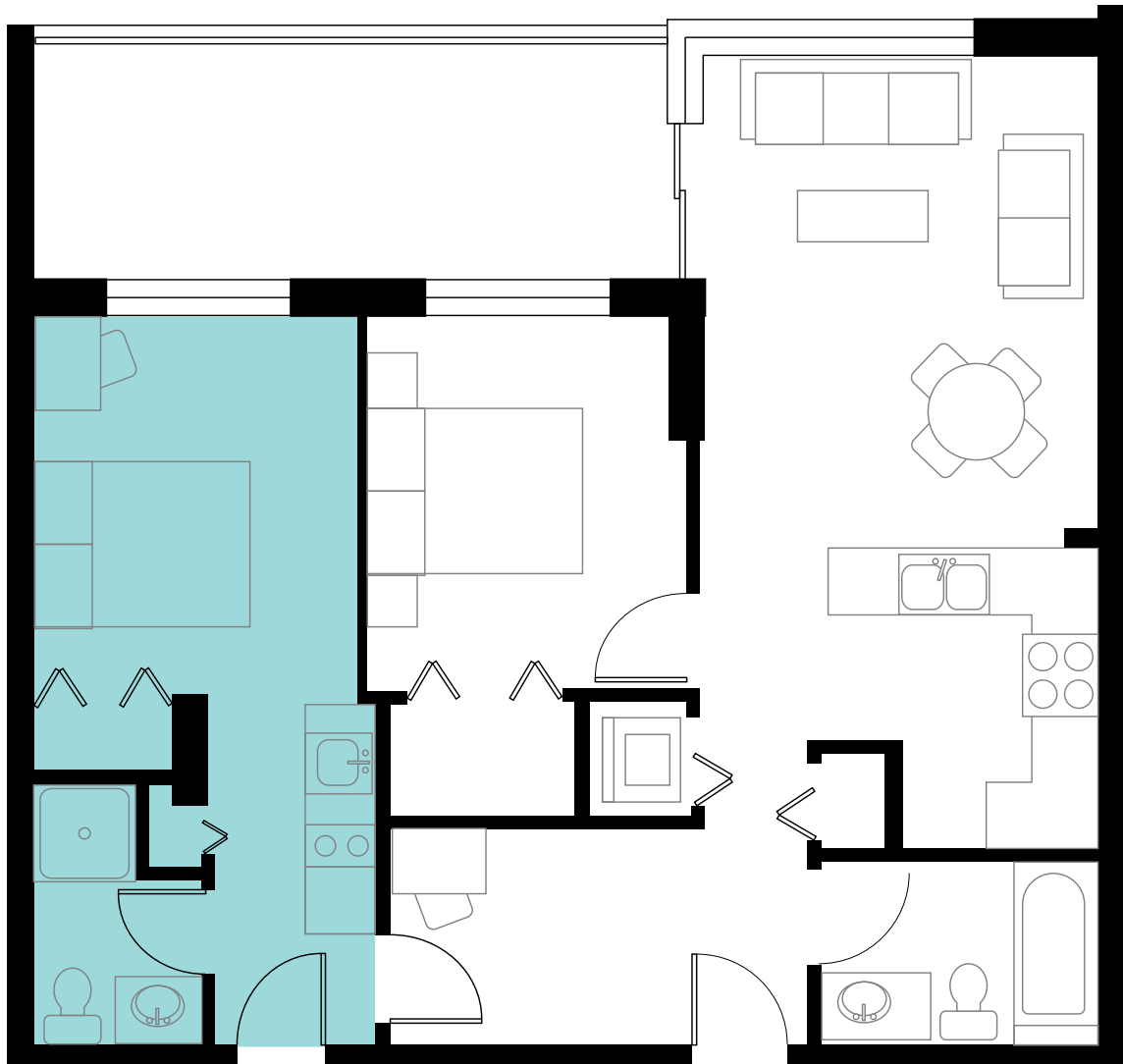
Floor plan of lock-off suite. Credit: Perkins & Co.
